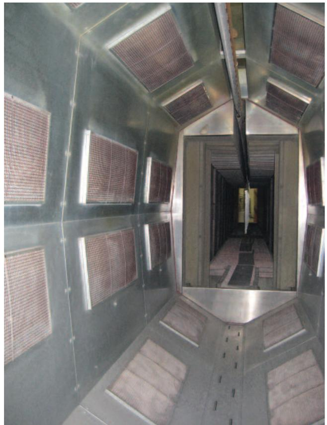
Greco Aluminum Railings’ pre-gel oven interior shows the catalytic IR heaters strategically positioned to blanket the entire part. The interior of the curing oven is also evident here.
