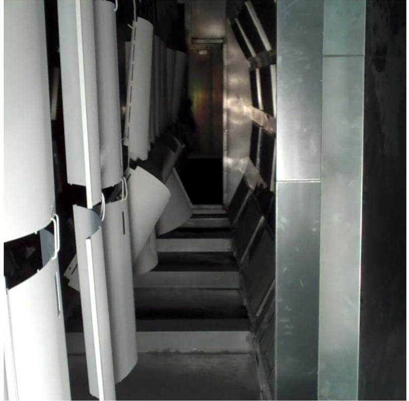
Once the testing was complete and the oven design established, the powder Pre-gel ovens using the gas catalytic infrared heaters were quoted. The Visioneering Pre-Gel oven is 24 ft. long and has 8 zones of control.
